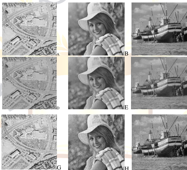
Fig. 5 Performance analysis of Presented Compression Technique: Original Image (A) Ariel, (B) Girl, (C) Boat; Compressed Image using DCT (D), (E) and (F); and Compressed Image using DWT (G), (H), and (I)
